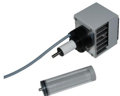
Remove the transparent condensate trap by slipping it out of gasket.
