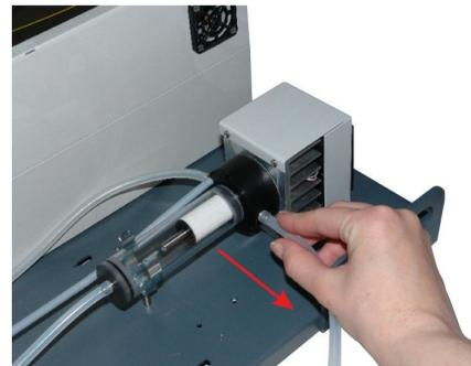
Disconnect the tubing that feeds the gas to the dryer.
