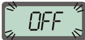
Picture 61. While the additional channel is being ventilated the device displays the **OFF** note and the last measured value in turns.
