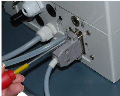
Disconnect the electric cable between the analyser and the gas dryer.
