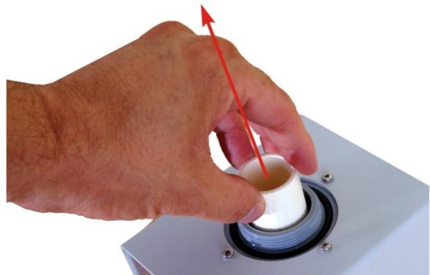
Picture 55. Replacement of filter inlet in MD3 gas dryer.
