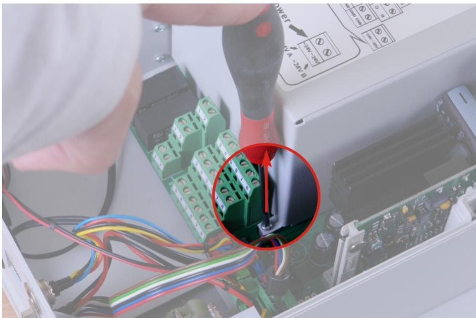
Picture 48. Metal cover – location of holding screw.
