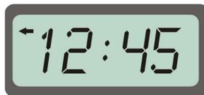
Picture 57. Example of the first display reading (*display #1*) during the "**WARMING-UP**" or "**STAND-BY**" stages.
